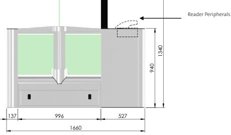
$Concrete\ Base\ to\ specification\ at\ least\ (cube)\ 300N/mm^2\ of\ resistance.\ Base\ to\ be\ flat\ and\ level\ to\ +/-\ 5mm\ over\ footprint\ area.$
