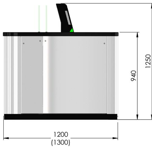
Concrete Base to specification at least (cube) 300N/mm<sup>2</sup> of resistance. Base to be flat and level to +/- 5mm over footprint area.
